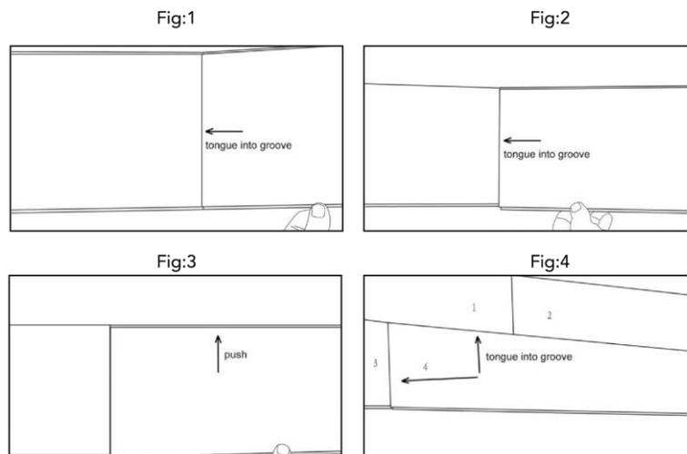
7. To start the second row, cut a plank that is at least 15cm shorter than the first plank in the first row (you may use the left over from the last plank of the first row). Then install this first plank by inserting the long side tongue into the groove of the plank in the first row.
